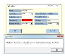
Note that once you select the Header, SS 1.0 will calculate and display the dew point temperature for that header. If the steam production from this boiler is known, then enter this flowrate in the Outlet Flowrate box. If SS 1.0 is to solve for this flowrate, then leave it blank, but remember, you can only have one unknown.
