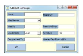
Inlet Header. Select the Header supplying steam to the heat exchanger. Note that once you make your selection, SS 1.0 will calculate and display the dew point temperature of the selected header.
